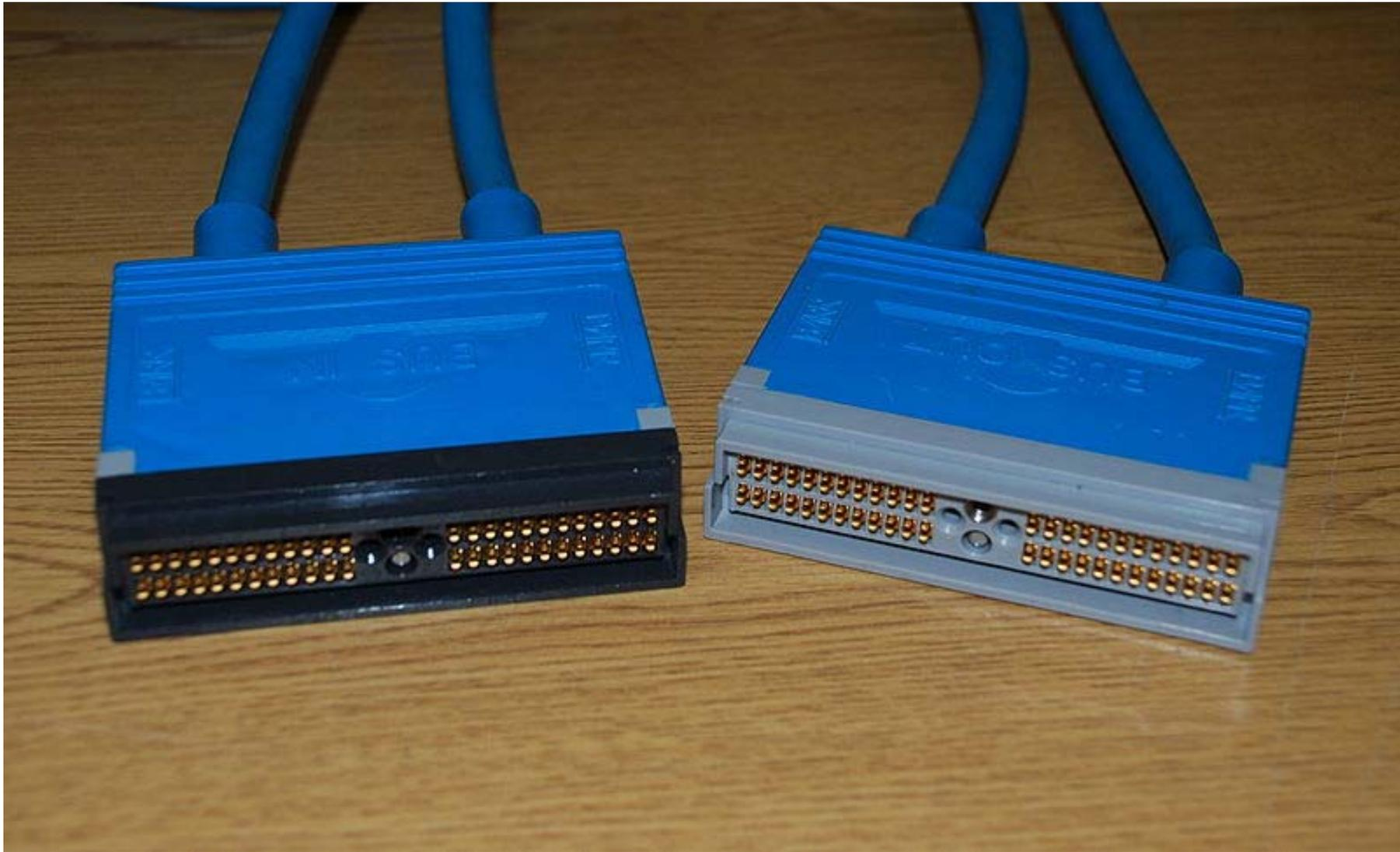
**Parallel Channel Bus- and Tag Cable Connectors,
