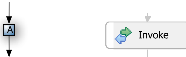
Figure 6.5.: An ACTIVITY node of the PFG and the possible representation in BPEL
